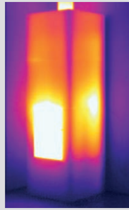
3 hour after heating Average surface temperature 88 °C
