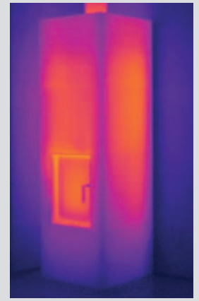
12 hour after heating Average surface temperature 45 °C
