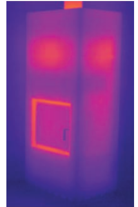
8 hour after heating Average surface temperature 46 °C
